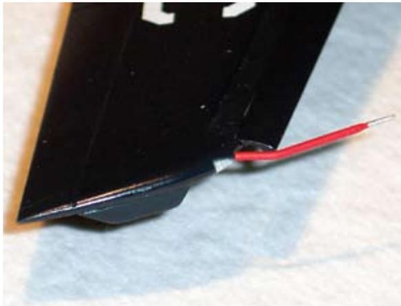
fied to a Navy-style gear with a fork around the nose wheel. But the biggest difference was the length. The gear was noticeably longer to increase the Fury's angle of attack during takeoff. I viewed the DVD and references several times to come up with a new gear design. The kit gear was cut off just above the oleo and a .020 in. brass rod made for the new oleo.
