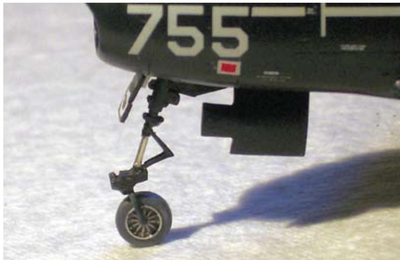
Bill cut the kit nose gear strut and added a new oleo and a set of styrene anti-torque scissors.
