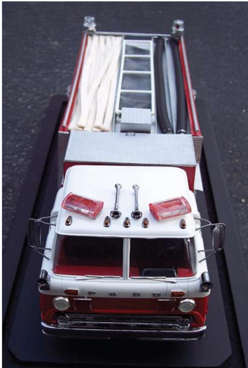
The brackets for the rear-view mirrors were far too thick, so Ed used thin solder to replace them.
